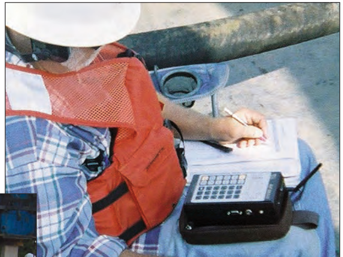
E-Saximeter with antenna receives energy and depth data from wireless transmitters.
