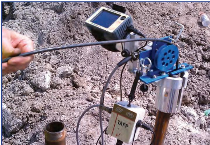
Thermal Integrity Profiler (Probe System).
